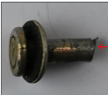
Photo No. 4: 8.5 mm section of the flathead pin from L/H Main Landing Gear.
