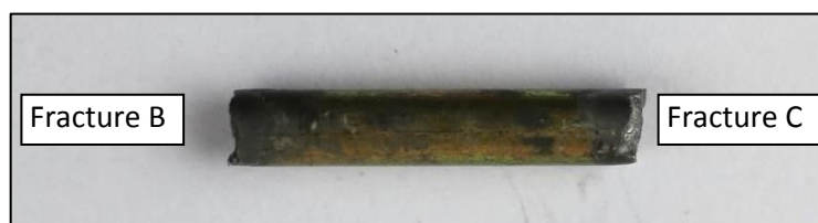
Photo No. 6: 16 mm long section of flathead pin removed from migrated L/H shock absorber pin.
