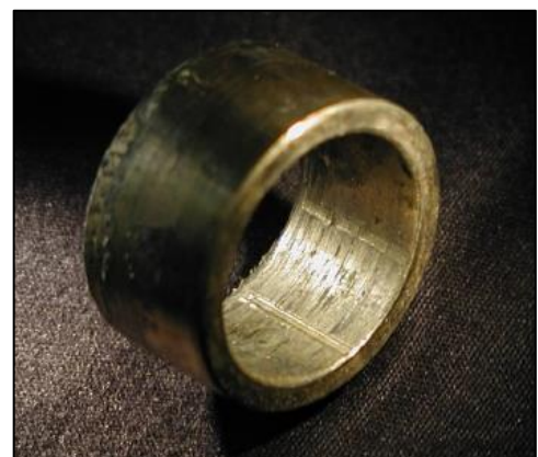
Photo No. 10: Scoring on RHS bushing (with bushing removed).
